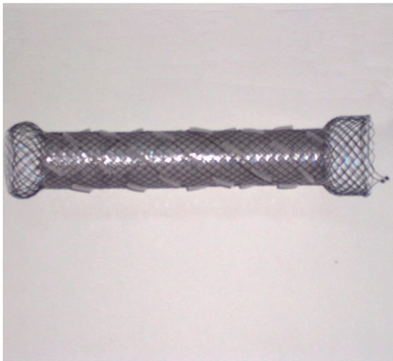
Figure 1: Covered self-expandable esophageal stent with plastic sheaths holding 125 I seeds fixed on outside of stent (arrows).
